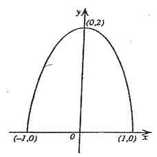
An ornamental arch window 2 metres wide and 2 metres high is to be made in the shape of an arc of either a cosine curve or a parabola, as illustrated on axes above.
