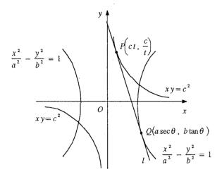
The line l is a common tangent to the hyperbolas  $xy = c^2$ ,  $\frac{x^2}{a^2} - \frac{y^2}{b^2} = 1$  with points of contact P and Q respectively.
