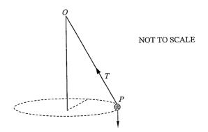
(i) Resolve the horizontal and vertical forces at P and show that  $\tan \theta = \frac{v^2}{rg}$  where r is the radius of the circle.
