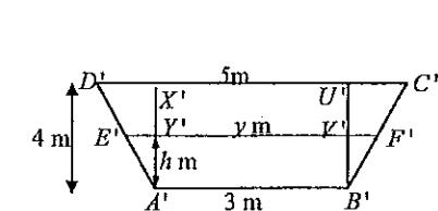
Cross-sections parallel to the base of the trench will be rectangles with sides  $x$  and  $y$  as shown in diagrams above.
