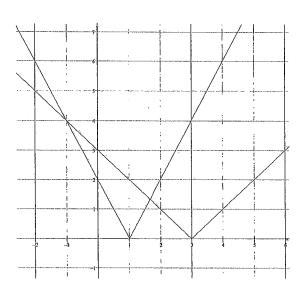
From the graph, the intersections occur when both branches of y = |2x-2| cuts the negative branch of y = |x-3|.
