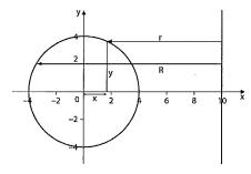
Slices are taken perpendicular to the axis of rotation (x=10). The base is an annulus.
