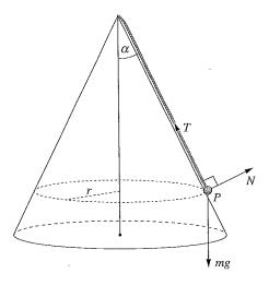
The forces acting on the particle are the tension, T, in the string, the normal reaction, N, to the cone and the gravitational force mg.
