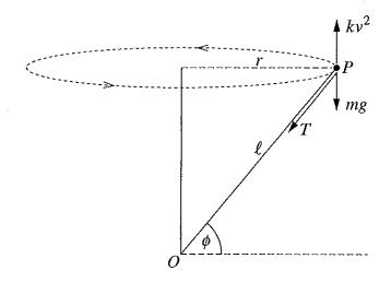
The forces acting on the aeroplane are the gravitational force mg, the tension force T in the string and a vertical lifting force  $kv^2$ , where k is a positive constant.
