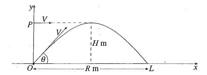
A particle is projected from a point O on horizontal ground with speed  $V \text{ m s}^{-1}$ at an angle of elevation of  $\theta$ , landing at L, as shown. You may assume that the displacements of this particle after t seconds are given by
