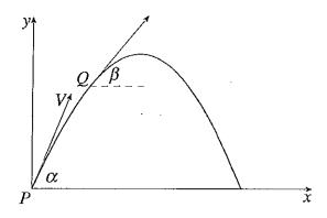
Its equations of motion are  $\ddot{x} = 0$ ,  $\ddot{y} = -g$ .
