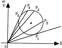
As P moves around the circle, the largest and smallest values of angle XOP will occur when OP is a tangent to the circle - at the positions P, and
