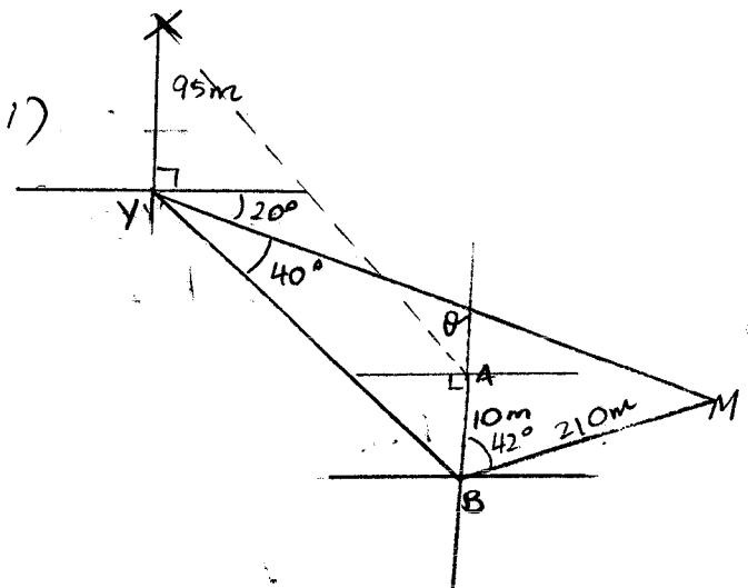
$$\text{i)} \quad \theta = 90^\circ - 42^\circ \quad (\text{right } \angle = 90^\circ) \\ = 48^\circ$$
