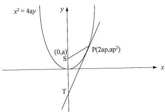
Point P(2ap,ap<sup>2</sup>) lies on the parabola  $x^2 = 4ay$  and S is the focus. The tangent at P meets the y-axis at T.
