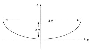
A satellite dish in the shape of a parabola has a diameter of 4 metres and a depth of 2 metres. Find the focal length of the dish.
