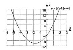
The parabola y = (2x - 1)(x + 4) has x intercepts x = -4 and  $x = \frac{1}{2}$ .
