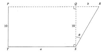
The vertical side of the gutter is 10 cm long and the other side is at an acute angle of  $\theta$  with the vertical. The sum of the three lengths in the gutter is 40 cm, i.e. 10 + a + RS = 40.
