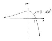
The diagram above shows the curve  $y = (1-x)e^x$ . There is a maximum turning point at (0,1).
