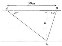
In the diagram above, two points A and B are 50 metres apart on the same side of a river. The point C is on the other side. A surveyor wants to determine the width w of the river. He measures  $\angle BAC$  to be 38° and  $\angle ABC$  to be 73°. Find the width of the river, correct to the nearest metre.
