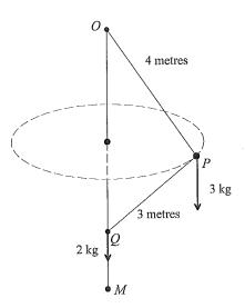
The above sketch shows a smooth vertical rod OM. Light inextensible strings OP and QP are attached to the rod at O and a mass of 3kg at P. At Q, a 2kg mass is free to slide on the rod. P is rotating in a horizontal circle about the rod.
