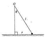
In the diagram a particle of mass m, attached to a string of length l, is suspended from a point O above a smooth, horizontal table with the string inclined at angle  $\theta$ to the vertical. The particle moves on the table with constant angular velocity  $\omega$  in a horizontal circle of radius r. The forces acting on the particle are the force due to gravity, the normal reaction N and the tension T in the string. Which of the following is an expression for T?
