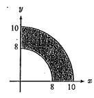
Use the formula:  $R = \frac{\pi}{4}(r_1 + r_2)(r_1 - r_2)$  where  $r_1$  is the outer radius and  $r_2$  is the inner radius, to calculate R, the area of the part annulus.
