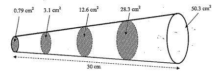
A number of circular cross sections at equal distances along the length of the container are shown with areas calculated.
