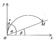
A ball is thrown from O with initial velocity v and angle  $\alpha^o$  to the horizontal. A fixed straight road passes through O and is on an incline to the horizontal at angle  $\beta^o$ , where  $\alpha > \beta$ . The ball hits the road at M.
