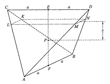
In the diagram, AB and CD are line segments of length 2a in horizontal planes at a distance 2a apart. The midpoint E of CD is vertically above the midpoint F of AB, and AB lies in the South-North direction, while CD lies in the West-East direction.
