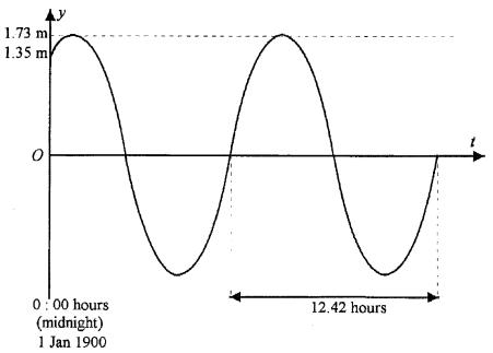
The diagram shows the tidal effect due to the Moon at Port Hedland on 1 January 1900. The water level can be approximated by a sine curve of the form  $y = A \sin(at + b)$  where y is the water level i metres measured as on the diagram and t is the time in hours after 0:00 hours.
