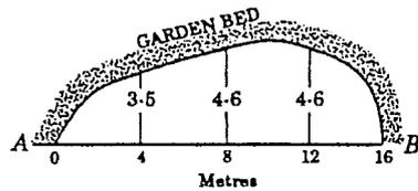
A section of grass between a path ( $AB$ ) and a curved garden bed is to be removed, and concrete to a depth of 10 cm is to be laid.
