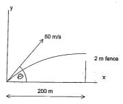
A ball is hit at 50 m s<sup>-1</sup>. The fence 200 metres away is 2 metres high. You may neglect air resistance and acceleration due to gravity can be taken as  $10 m s^{-2}$  and you may assume the following equations of motion  $x = 50 t \cos \theta$  and  $y = 50 t \sin \theta - 5 t^2$
