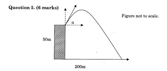
The diagram shows the path of a projectile launched at an angle of elevation  $\alpha$ , with an initial velocity of 40 m/s, from the top of a 50 metre high building. The acceleration due to gravity is assumed to be 10 m/s<sup>2</sup>.
