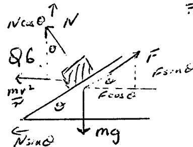
$$\begin{aligned}N \cos \theta + F_{\text{fricnt}} &= mg \\ \frac{mv^2}{r} &= N \sin \theta - F_{\text{fricnt}}\end{aligned}$$
