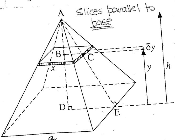
Slicing the pyramid parallel to its base gives square slices of side  $x$  and width  $\delta y$ , where  $y$  is the height of the slice above the base. E, C are midpoints of the sides of the base and slice respectively.
