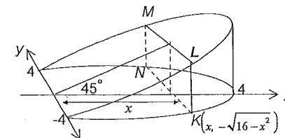
A rectangular slice  $KLMN$  is taken perpendicular to the base of the wedge at a distance  $x$  from the  $y$ -axis.
