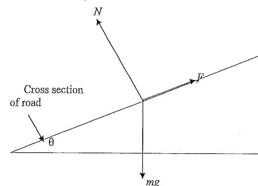
A road contains a bend that is part of a circle radius  $r$ . At the bend, the road is banked at an angle  $\theta$  to the horizontal. A car travels around the bend at constant speed  $v$ . Assume that the car is represented by a point of mass  $m$ , and that the forces acting on the car are the gravitational force  $mg$ , a sideways friction force  $F$  (acting up the road as drawn) and a normal reaction  $N$  to the road.
