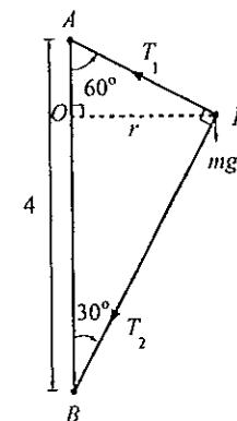
The forces acting on the particle at  $P$  are  $T_1$  (the tension in the rod  $AP$ ),  $T_2$  (the tension in the rod  $BP$ ) and  $mg$  (gravity).
