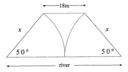
A bridge spans a river, and the two identical sections of the bridge, each of length x metres, can be raised to allow tall boats to pass. When the two sections are fully raised, they are each inclined at  $50^{\circ}$  to the horizontal, and there is an 18 metre gap between them, as shown in the diagram above. Calculate the width of the river in metres, correct to one decimal place.
