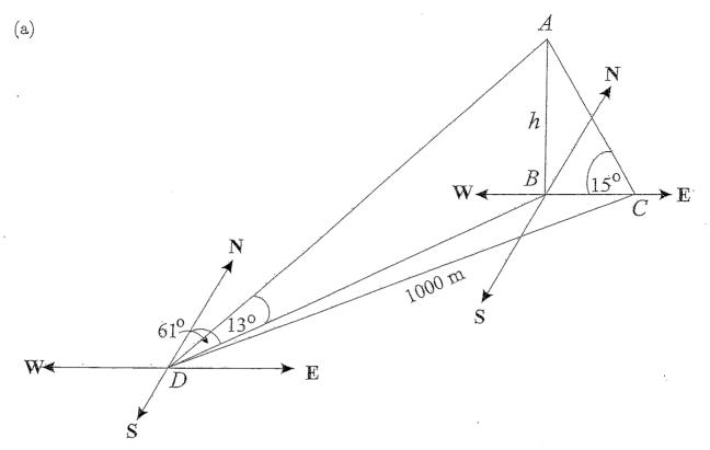
In the diagram above, AB represents a tower of height h metres. The angle of elevation of the tower from a point C due east of it is 15°. From another point D, the bearing of the tower is  $061^{\circ}\text{T}$  and the angle of elevation is  $13^{\circ}$ . The points C and D are 1000metres apart and on the same level as the base of the tower.
