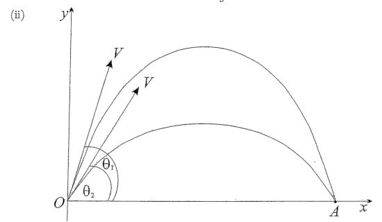
In the diagram above, two particles are projected from the origin with the same velocity V at different angles of projection  $\theta_1$  and  $\theta_2$ . They strike the same point A, on the horizontal plane through the point of projection, at times  $T_1$  and  $T_2$  respectively.
