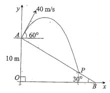
The diagram above shows a plane inclined at  $30^{\circ}$  to the horizontal, meeting level ground at B. A ball is projected from a point A on the plane, 10 metres above the horizontal. The angle of projection is  $60^{\circ}$  to the horizontal and the initial speed of the ball is  $40 \,\mathrm{m/s}$ .
