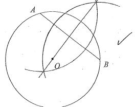
Construct the perpendicular bisector of the chord AB, clearly showing all construction lines.
