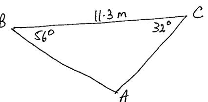
$\angle BAC = 92^\circ \quad (180^\circ - 56^\circ - 32^\circ)$ $\therefore \frac{AC}{\sin 56^\circ} = \frac{11.3}{\sin 92^\circ}$ $AC = \frac{11.3 \times \sin 56^\circ}{\sin 92^\circ}$ $= 9.37 \text{ m} \quad (2 \text{ d.p.})$ $(9.373834857\dots)$ | (1)<br>(1)<br>(1) |                   |
