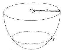
In the diagram above, a particle P is moving with constant speed v in a horizontal circle on the smooth inner surface of a hemisphere of radius OP=a. The force exerted by the hemisphere on the particle equals twice the weight of the particle. Let the acceleration due to gravity be g.
