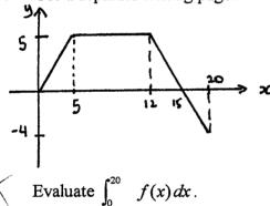
The diagram shows the (3) function y = f(x) between x = 0 and x = 20.
