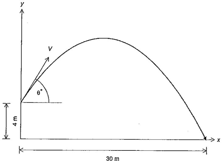
A rock is projected with a speed  $V \text{ ms}^{-1}$  from a point 4 metres above a flat sea. The angle of projection to the horizontal is  $\theta$ , as shown. Assume that the equations representing the acceleration of the rock are  $\ddot{x}=0$  and  $\ddot{y}=-10$ .
