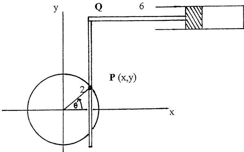
A piston moves back and forth on the end of a 6metre shaft.
