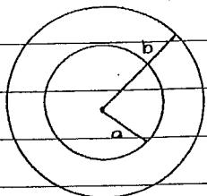
$$\begin{aligned}\text{Area annulus} &= \pi b^2 - \pi a^2 \\ &= \pi(b^2 - a^2) \\ &= \pi(b-a)(b+a)\end{aligned}$$
