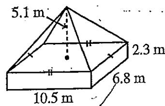
$$V = \frac{1}{3} \times (10.5 \times 6.8) \times 5.1 + 10.5 \times 6.8 \times 2.3 \\ = 285.6 \text{ m}^3$$
