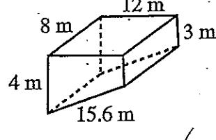
$$\begin{aligned} &\frac{1}{2} \times 12 (3+4) \times 8 \\ &= 336 \text{ cm}^3 \end{aligned}$$
