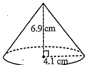
$$\begin{aligned} V &= \frac{1}{3} \times (\pi \times 4.1^2) \times 6.9 \\ &= 121.5 \text{ cm}^3 \end{aligned}$$
