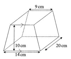
A special container has dimensions as shown above. The shape of the front end is a trapezium.
