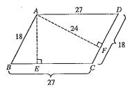
Area of parallelogram ABCD=  $BC \times AE = CD \times AF$  $27 \times AE = 18 \times 24$
