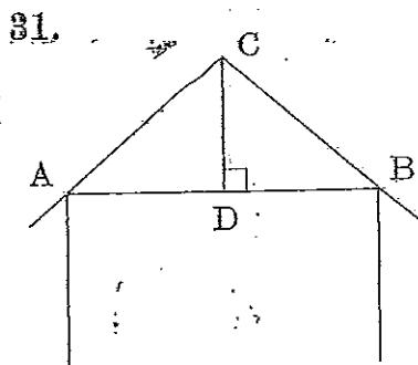
The roof of a house is in the shape of a triangle when viewed from the side. If the width of the house AB is 24 m and the height of the roof is 8 m, calculate the slant height BC of the roof. It can be assumed that the perpendicular height CD is in the centre of AB.
