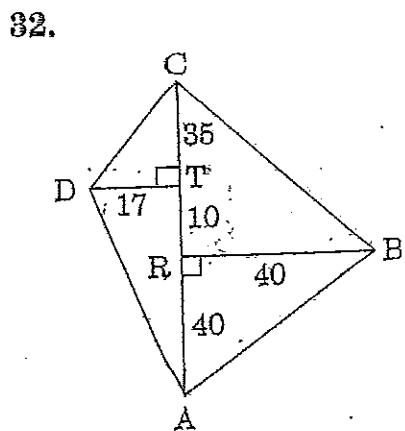
A surveyor makes this sketch of a paddock in his note book. The measurements are  $AR = 40$  m,  $RT = 10$  m,  $TC = 35$  m,  $DT = 17$  m,  $RB = 40$  m. Calculate the perimeter of the paddock correct to the nearest metre.
