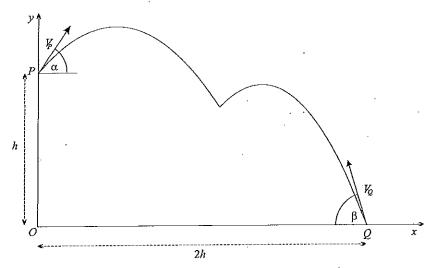
(i) For the particle launched from P, the acceleration equations are  $\ddot{x}_P = 0$  and  $\ddot{y}_P = -g$ . Show that at time t seconds, the respective horizontal and vertical distances from O,  $x_P$  and  $y_P$  are:
