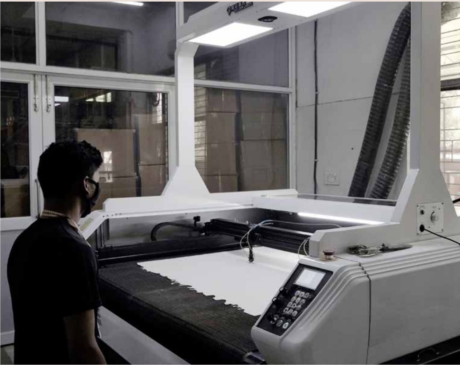
State-of-the-art optical laser cutting recognizes motifs and cuts around them to give us new ways of making precise applique products.
