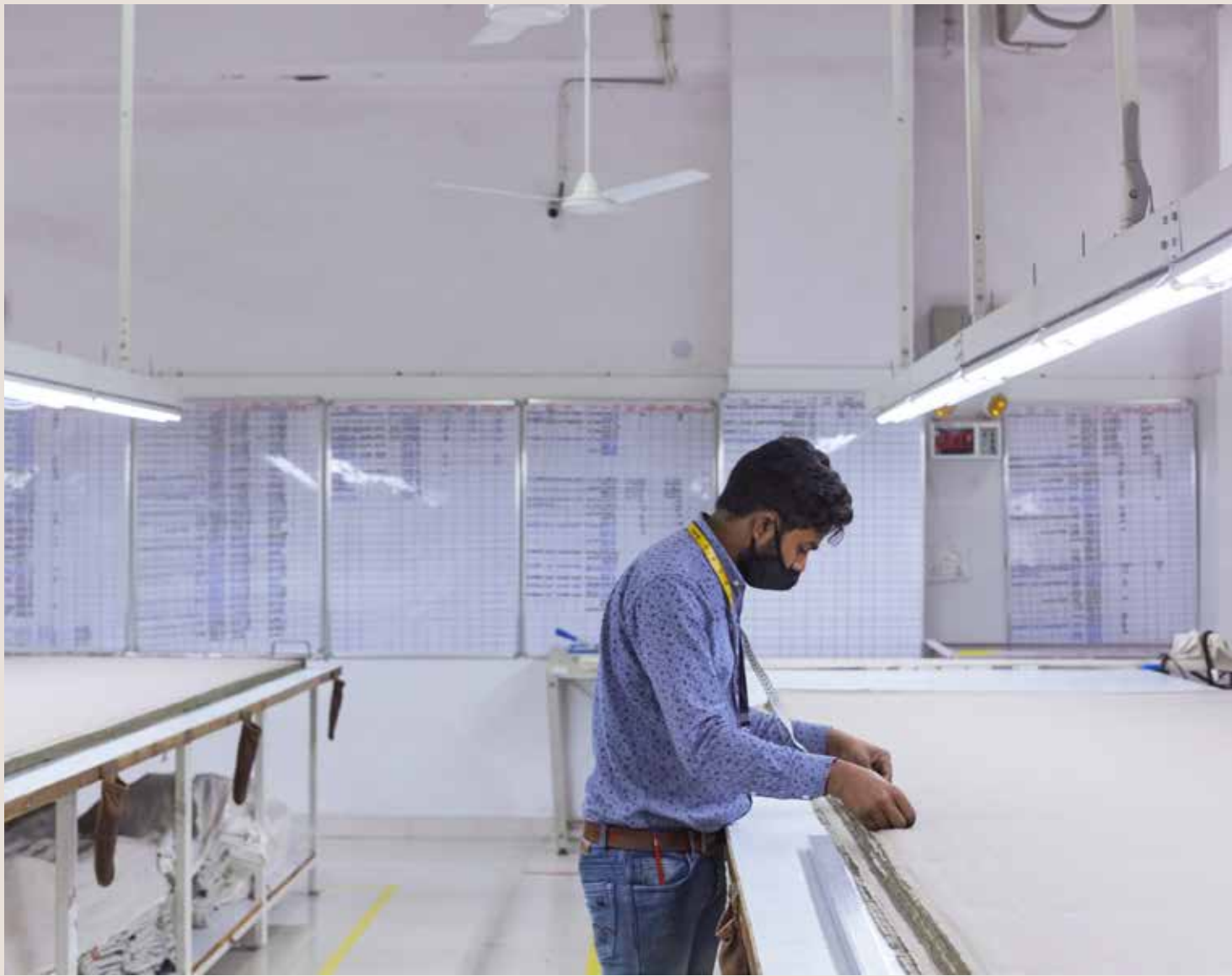
Cutting is where it all starts - patterns are marked with precision and the fabric is layered to be cut into panels for embroidery and stitching
