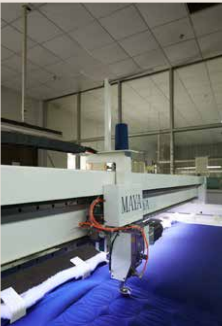
State-of-the-art optical laser cutting recognizes motifs and cuts around them to give us new ways of making precise applique products.
