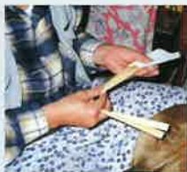
Nakatuke (insert the bamboo sticks between the surface papers)
