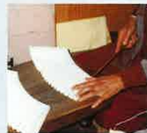
Nakasashi (insert bamboo wires between the papers)
