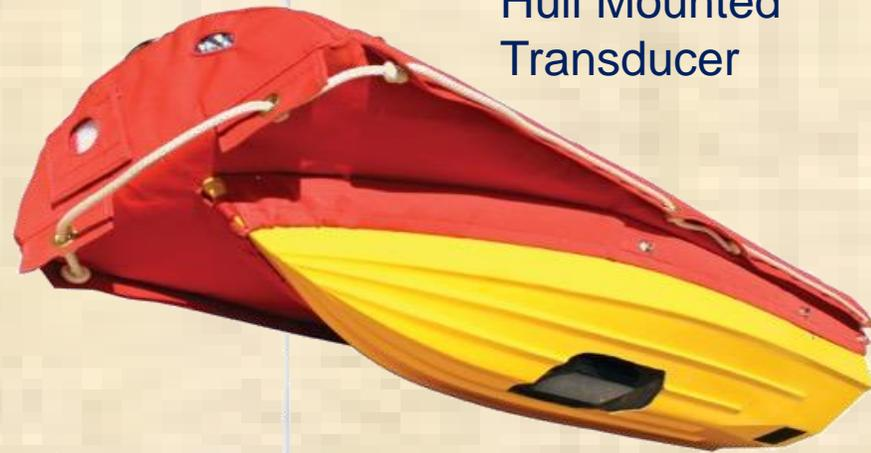
Hull Mounted Transducer
