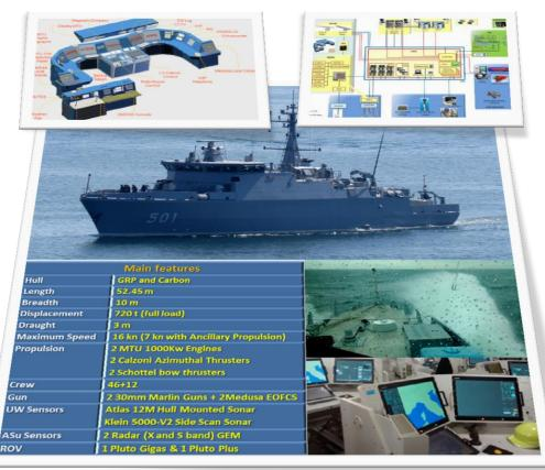
The MH&PV program provides the supply of two Minehunters (with a third optional) and relevant services (Training, ILS) for a Foreign Navy.
