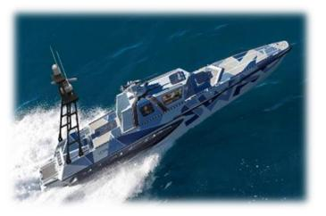
The SWAD is the result of a research project carried out by the SD division of Leonardo in order to achieve a USV with chasing, interdiction and attack capabilities in anti-piracy missions, thanks to its capacity to reach the high speed of 70 knots and the remotely controlled HITROLE® 12.7mm machine-gun.
